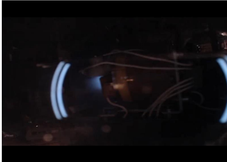
FIGURE 7: Transition from plasma bridging to ignition plume.
