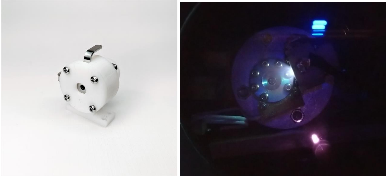
FIGURE 2: GDN1 full assembly (left) and operation of the GDN1 with Adamantane fuel on 2W neutralizer power (right).
