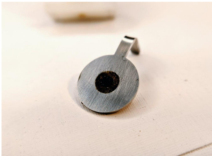
FIGURE 10: Significant amorphous carbon deposit on the anode plate of the neutralizer, clogging the neutralizer output.
