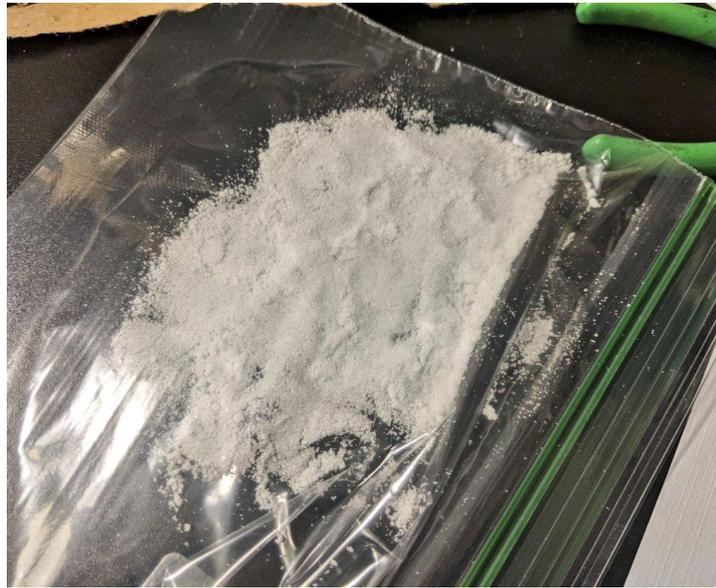
**FIGURE 2:** *Adamantane fuel preparation for loading into the test sublimation cell*
