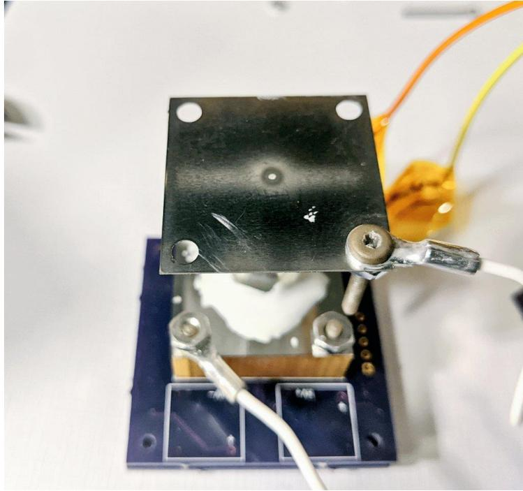
**FIGURE 11:** Plasma erosion around the output aperture of the ionization test cell
