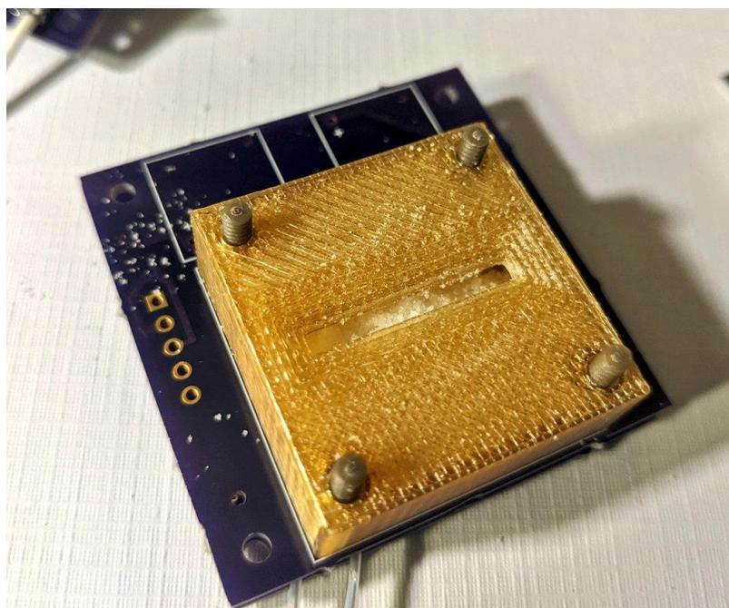
**FIGURE 5:** Loading of Adamantane fuel into the test sublimation cell housing
