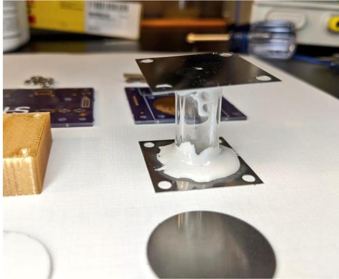
**FIGURE 6:** Ionization test cell made from stainless steel, borosilicate glass, and Hysol-1C epoxy
