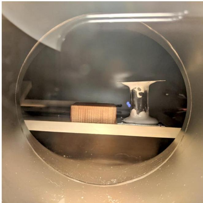
**FIGURE 7:** Vacuum baking and degassing of the Ultem fuel housing and ionization cell
