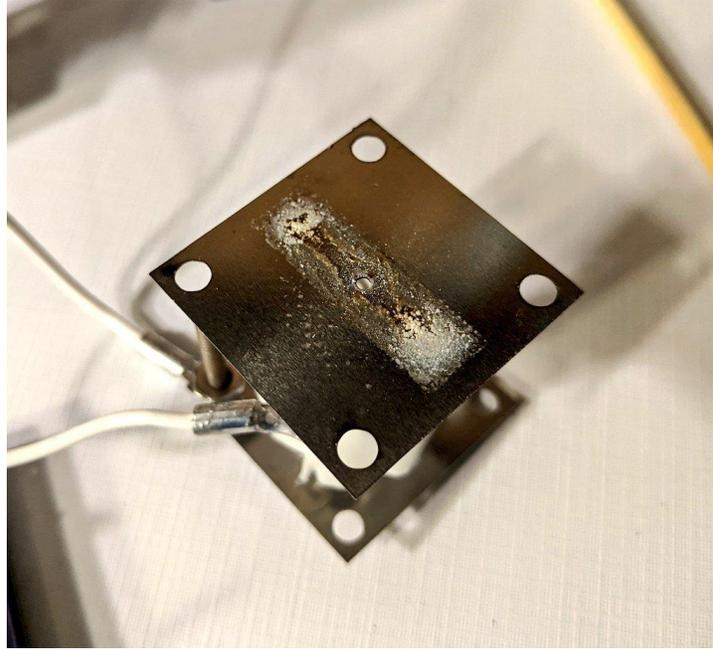
*FIGURE 13: Slight charring and buildup of Adamantane fuel on the bottom plate of the ionization test cell*
