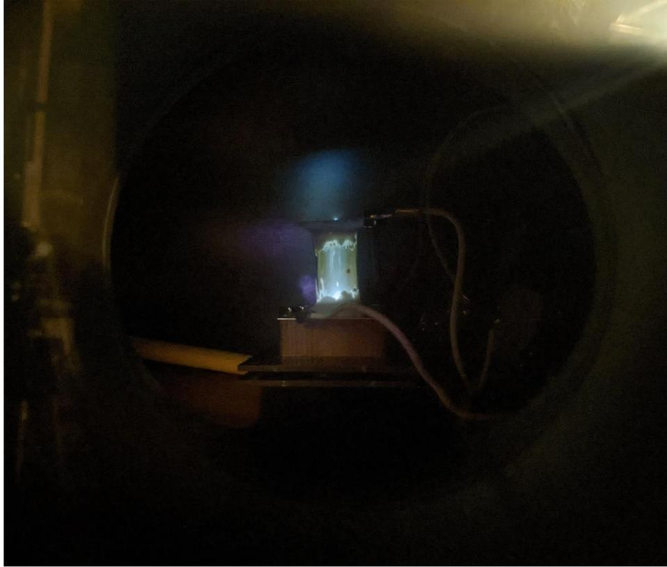
*FIGURE 10: Successful Adamantane plasma glow-discharge initiated at 2W discharge power and 3.5W sublimation heater power*
