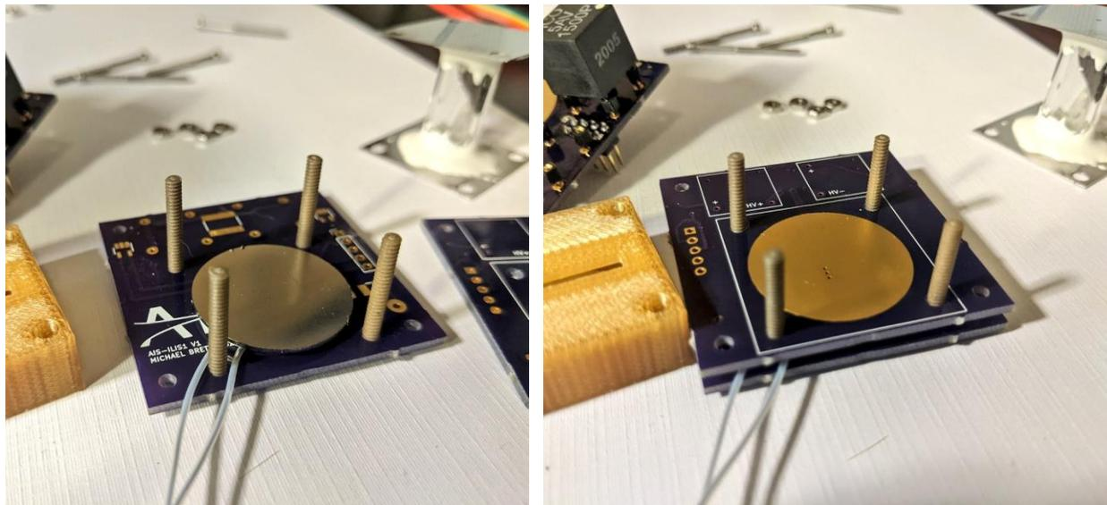
**FIGURE 4:** Heater assembly using ILIS1 boards, a ceramic-metal disc heater, and nickel contact plate
