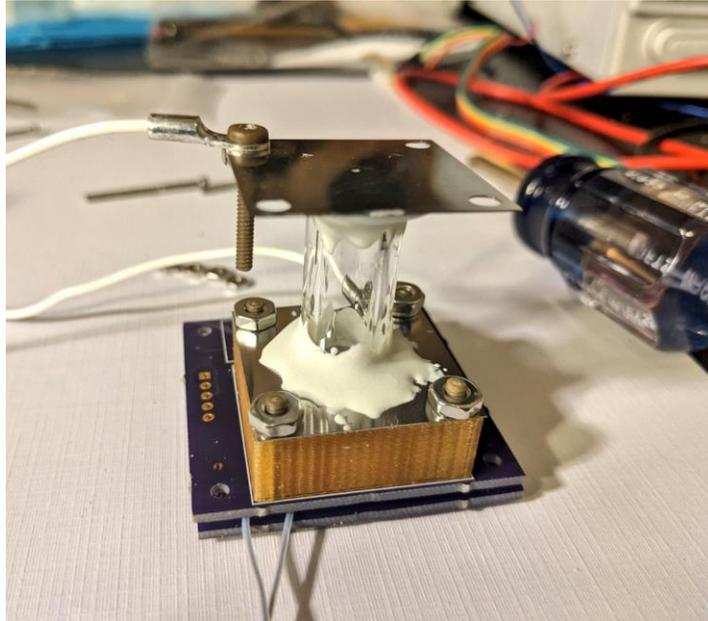
*FIGURE 8: Completed and assembled prototype sublimation and ionization test cell*
