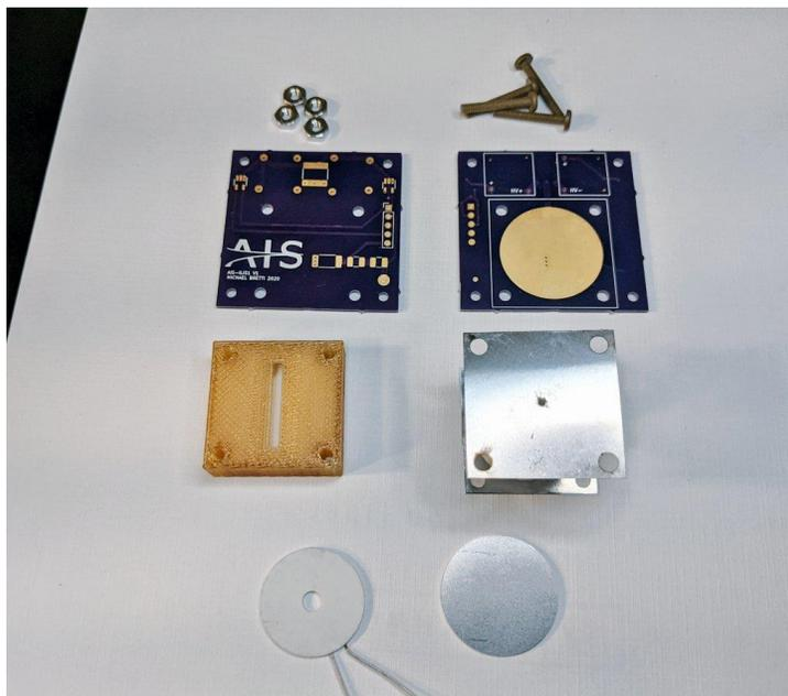
**FIGURE 3:** *Parts used for the sublimation and ionization test cell*
