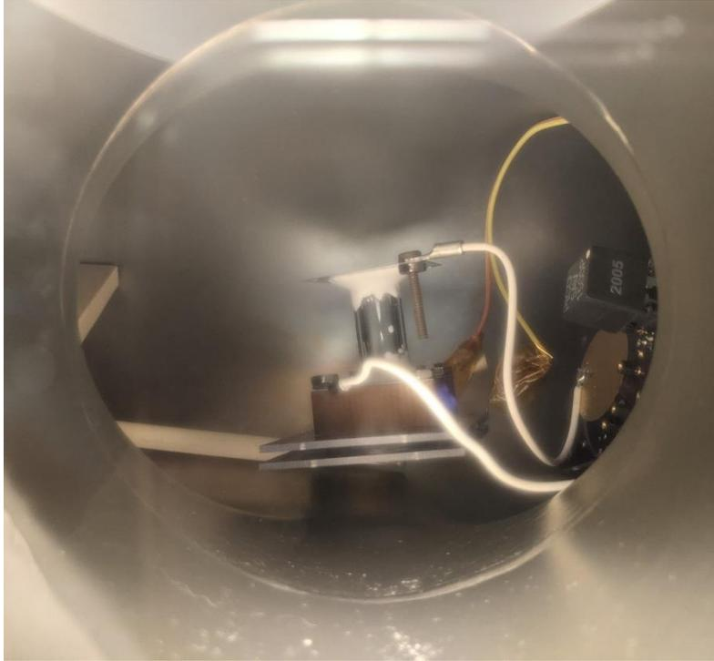
**FIGURE 9:** *Mounting of the test cell in the high vacuum chamber for testing*
