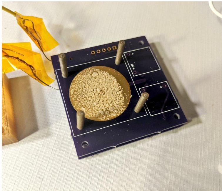
**FIGURE 12:** Near complete sublimation of the Adamantane fuel charge during the test
