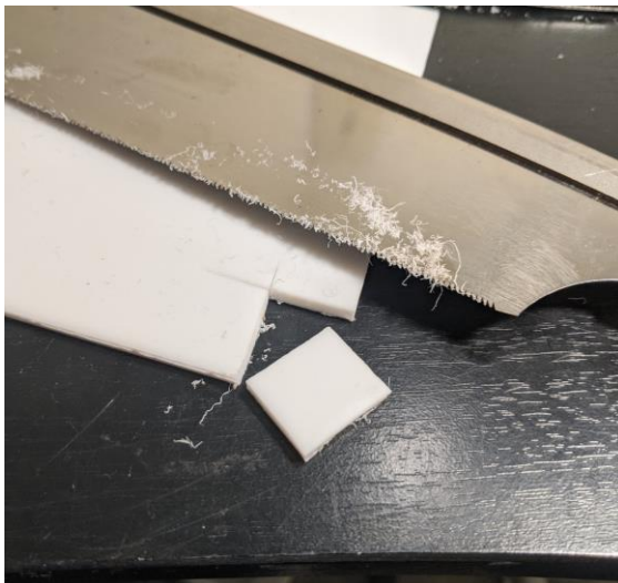
Figure 2 and 3: Modified 1/8" thick Teflon fuel plate
