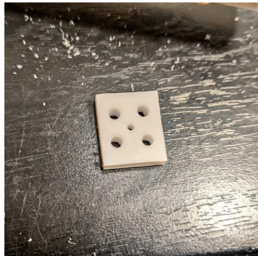
Figure 2 and 3: Modified 1/8" thick Teflon fuel plate
