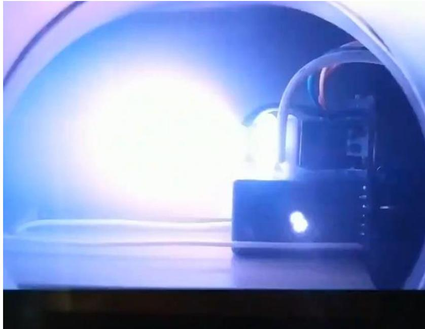
**FIGURE 25:** *Plasma plume during thruster operation*
