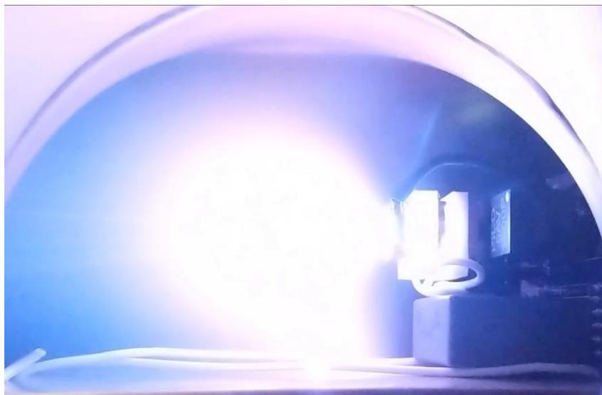
**FIGURE 10:** *gPPT3/EPPT1 firing in high vacuum at 3 Hz*
