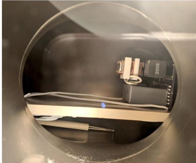
**FIGURE 9:** *Thruster mounting inside high vacuum chamber*
