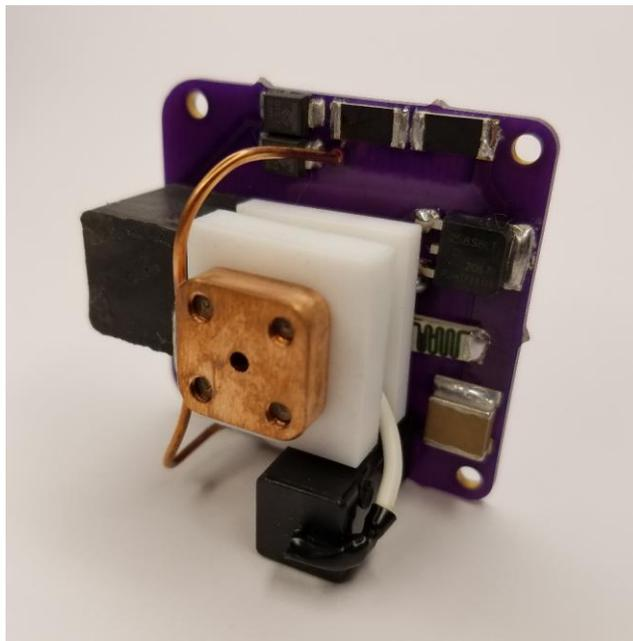
*FIGURE 2: Original AIS-gPPT3-1C micro pulsed plasma thruster module*
