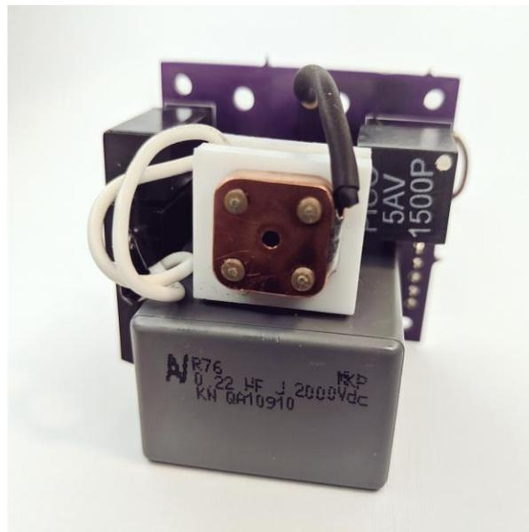
**FIGURE 11:** gPPT3/EPPT1 thruster assembly for ignition test 2
