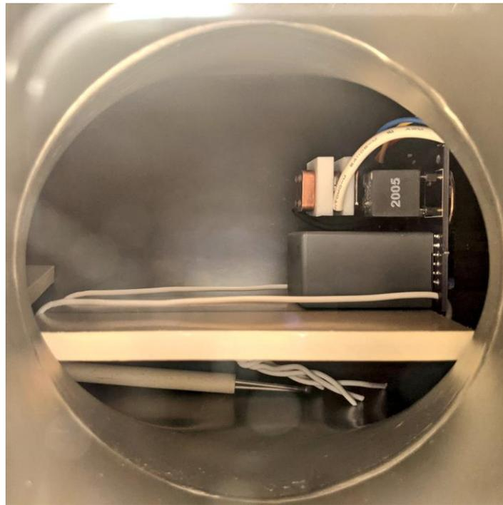
**FIGURE 19:** Thruster mounting inside high vacuum chamber
