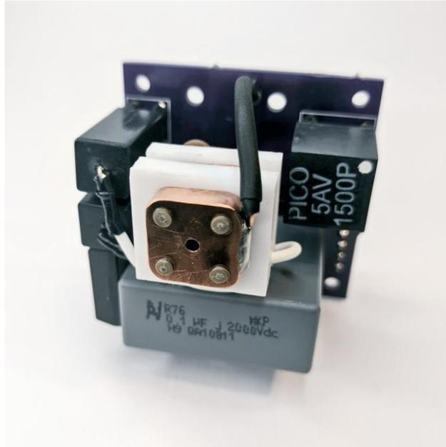
**FIGURE 8:** *gPPT3/EPPT1 prototype assembly for ignition test 1*
