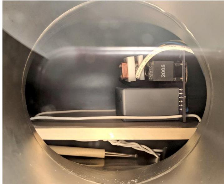
**FIGURE 22:** Thruster mounting inside high vacuum chamber
