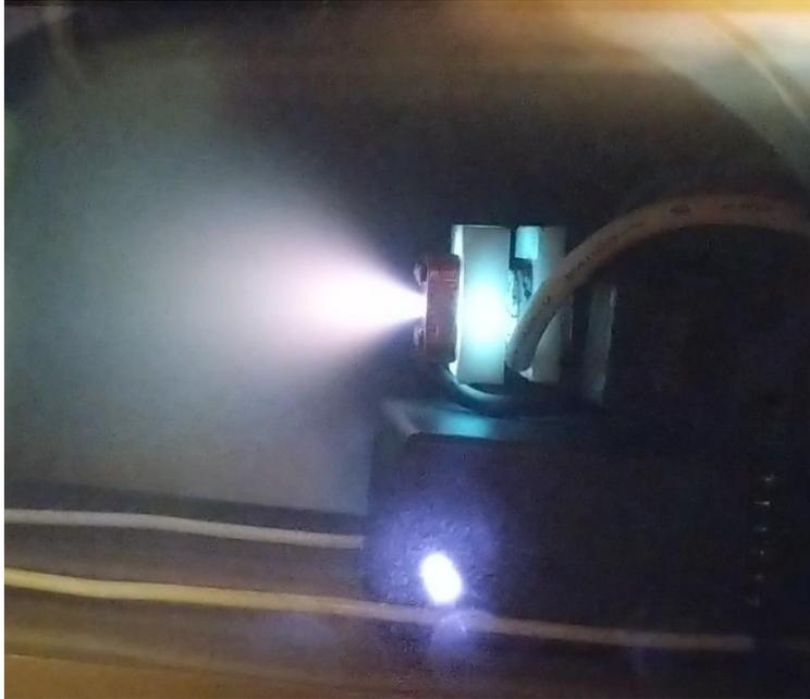
*FIGURE 23: Plasma plume during thruster operation with anode-side triggering and no magnetic nozzle*
