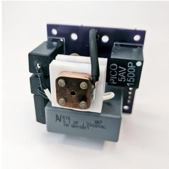
**FIGURE 1:** Completed gPPT3/EPPT1 prototype hybrid micro pulsed plasma thruster assembly
