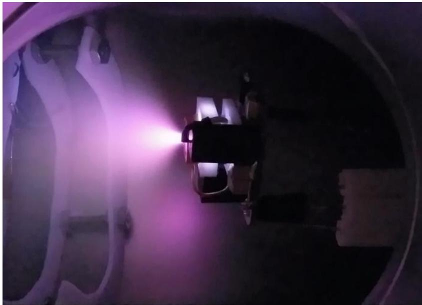
**Figure 4:** *AIS-gPPT3-1C plasma plume*
