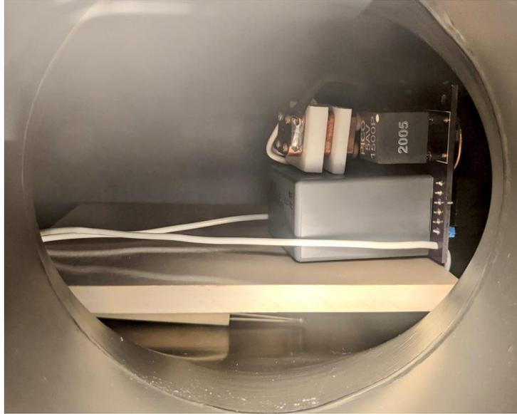
**FIGURE 12:** *Thruster mounting inside high vacuum chamber*
