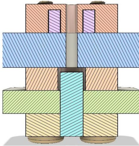
**FIGURE 3:** *gPPT3 thruster head cross-sectional view*
