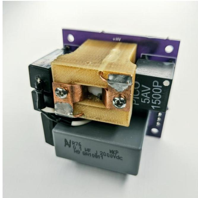
*FIGURE 5: Completed AIS-EPPT1 micro pulsed plasma thruster assembly*
