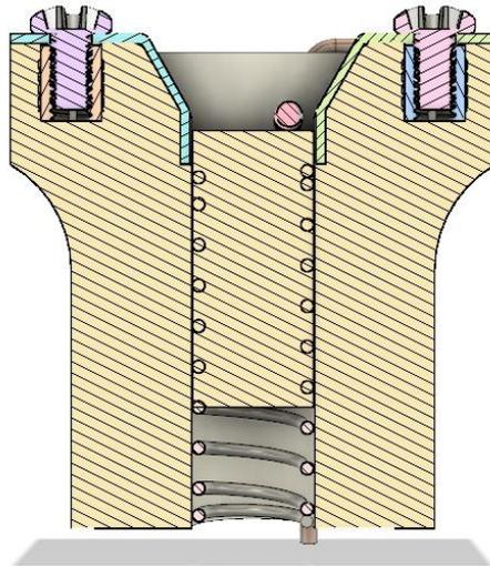
**FIGURE 6:** *EPPT1 thruster housing assembly cross-sectional view*
