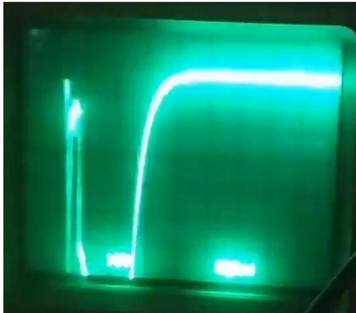
**FIGURE 21:** *Captured pulse during firing with extended 100uS pulse width discharge*
