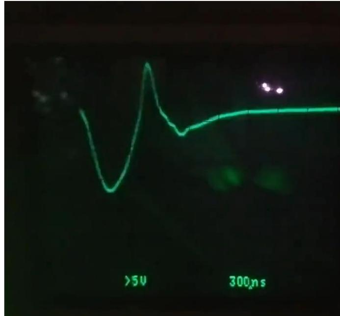
*FIGURE 26: Captured pulse during firing with typical 300ns pulse width discharge*
