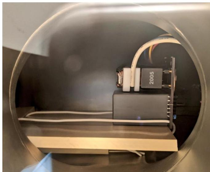
*FIGURE 24: Thruster mounting inside high vacuum chamber*
