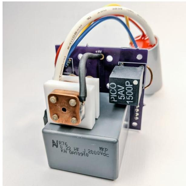
**FIGURE 14:** Front view of the gPPT3/EPPT1 modified prototype assembly for ignition test 3
