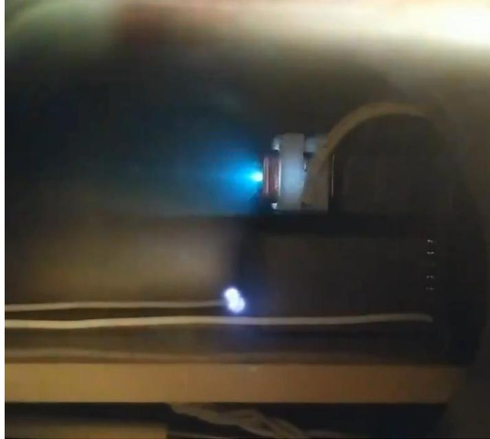
**FIGURE 20:** *Plasma plume during thruster operation with anode-side triggering*
