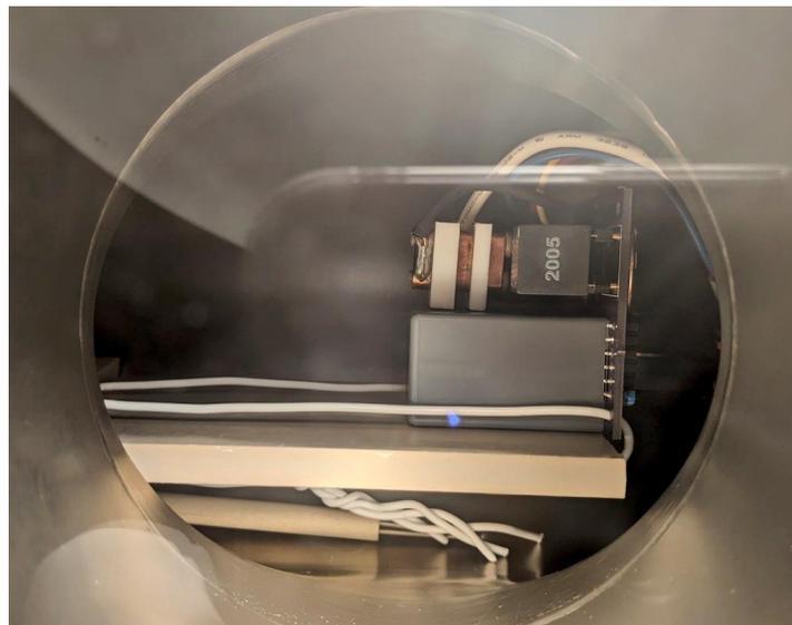
**FIGURE 16:** Thruster mounting inside high vacuum chamber
