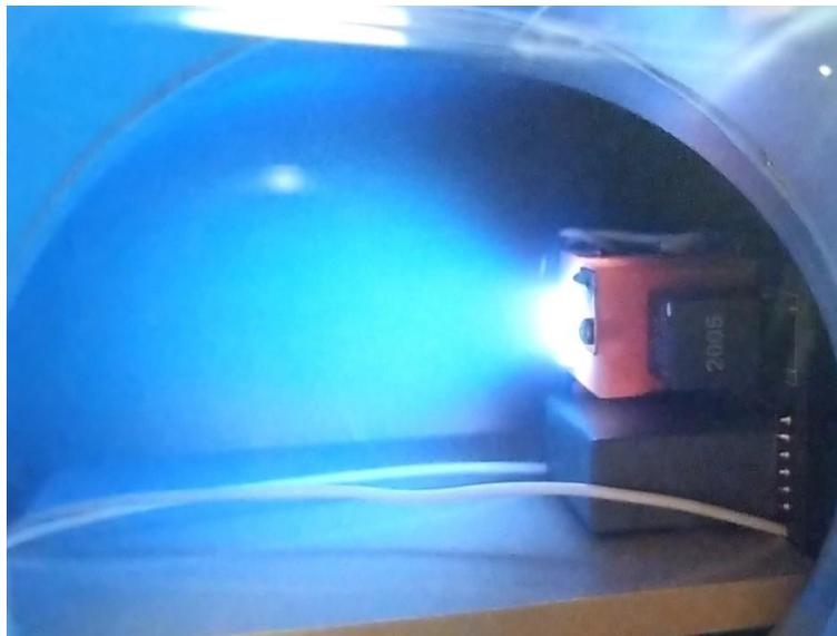
**FIGURE 7:** *AIS-EPPT1 plasma plume*
