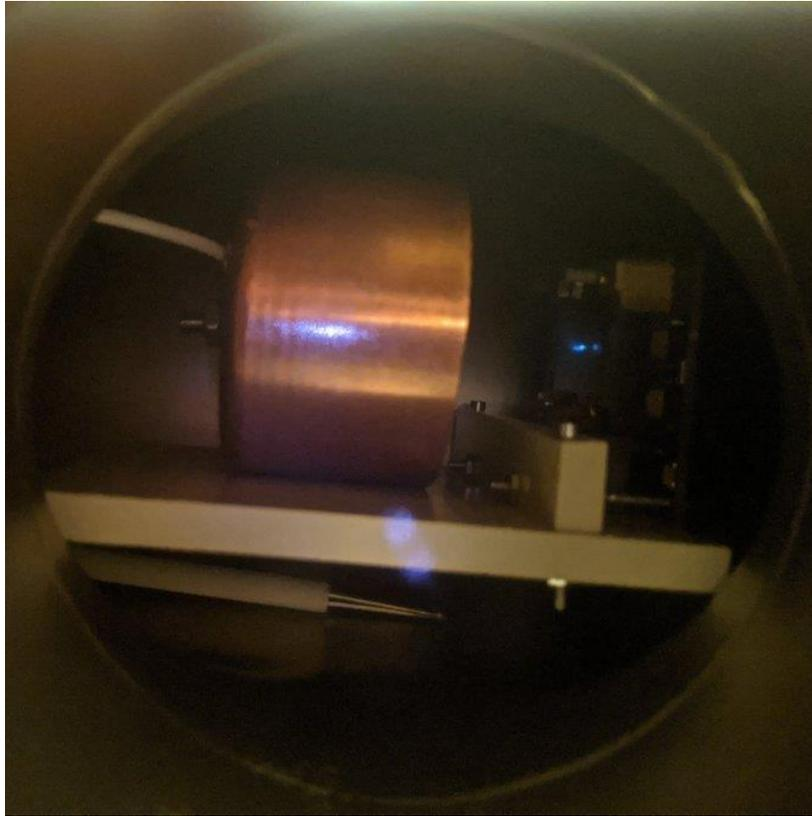
**FIGURE 6:** *Multisite ion beam emission at lower emission levels of 0.5uA*
