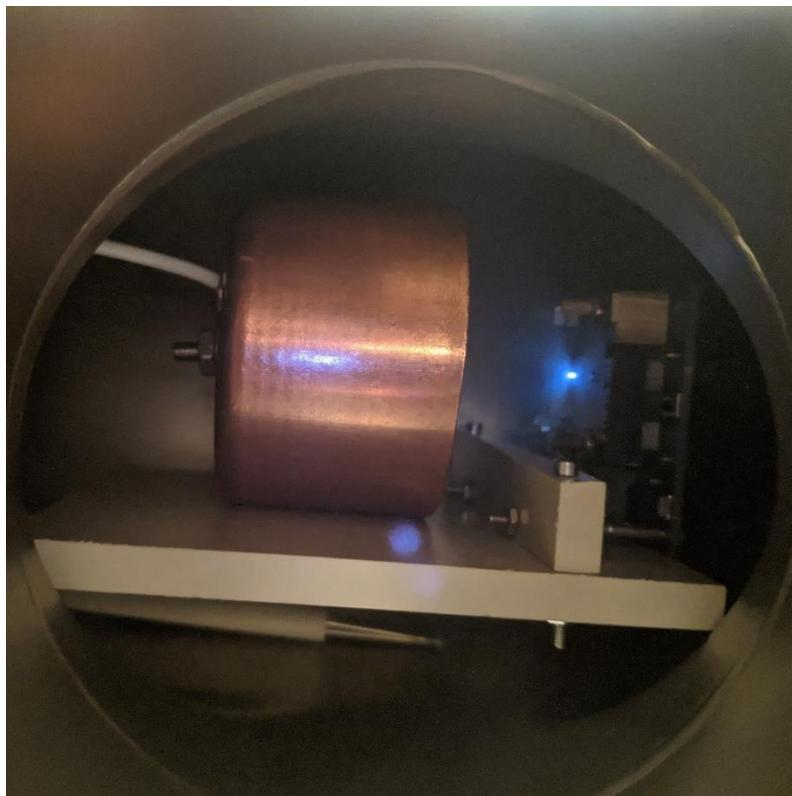
**FIGURE 5:** Ion beam emission at peak emission of 40uA, 3uN
