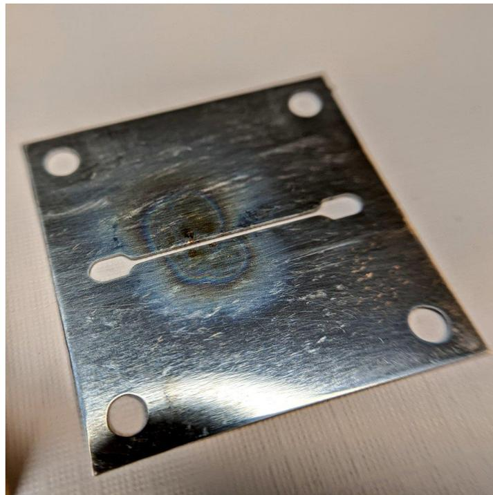
**FIGURE 9:** Close-up of the extractor plate. Evidence of beam impingement can be observed.
