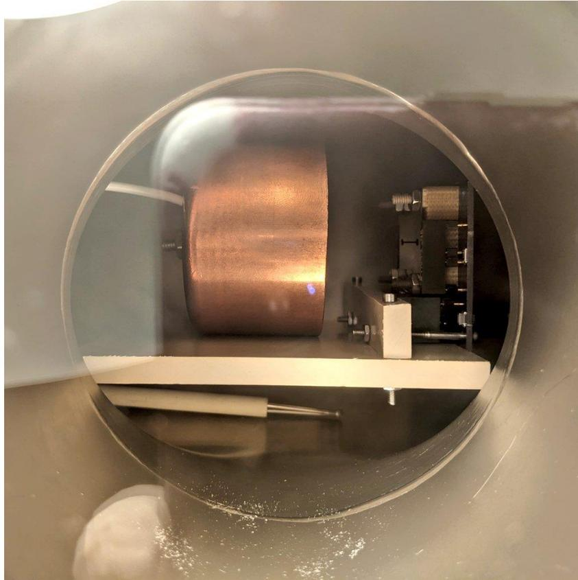
*FIGURE 4: ILIS1 and Faraday cup test stand mounted inside chamber*
