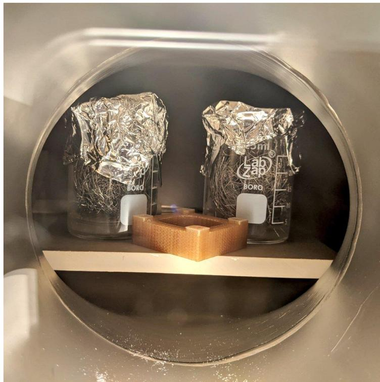
*FIGURE 3: Bakeout and degassing of the EMI-BF4 fuel, emitter, reservoir, and 3D printed thruster housing*
