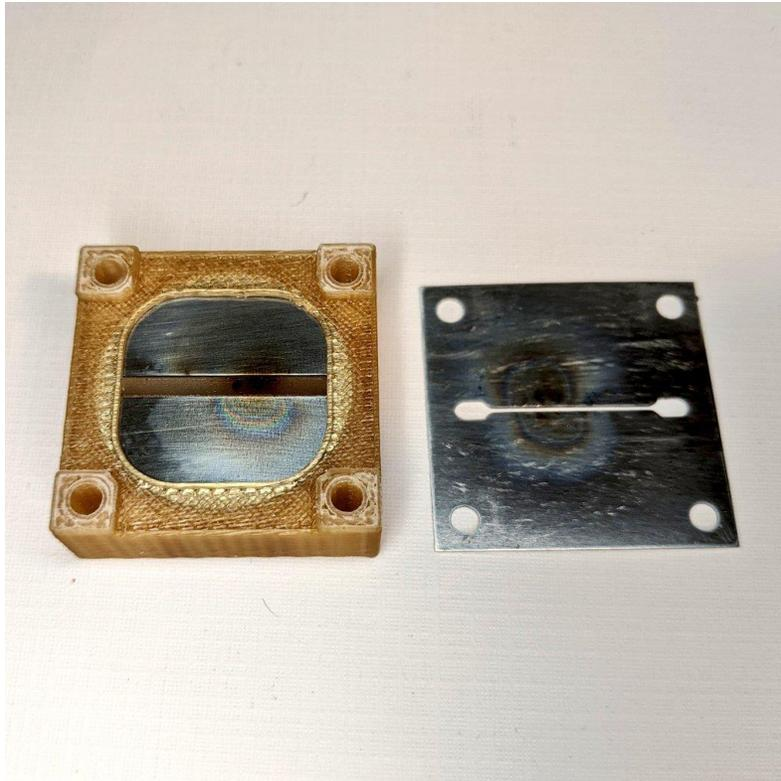
**FIGURE 7:** *Thruster assembly post-testing. Evidence of arcing, liquid bridging between the emitter and extractor, and beam impingement on the extractor can be seen.*
