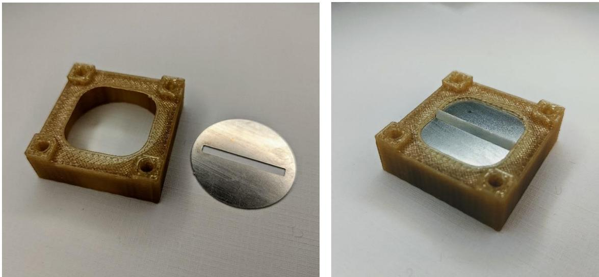
**FIGURE 2:** *New 3D printed housing design and shield electrode (LEFT), shield electrode with housing and test emitter for fit check (RIGHT)*
