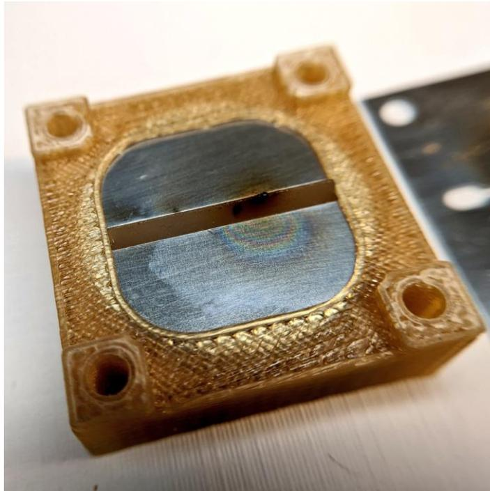
**FIGURE 8:** Close-up of the emitter, which shows evidence of charred fuel buildup at the peak of the emission site.
