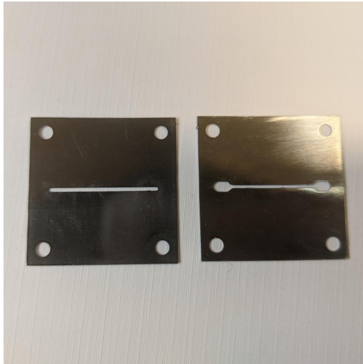
FIGURE 2: Original 0.75mm linear extractor (left) and new enhanced 0.5mm flared extractor (right)
