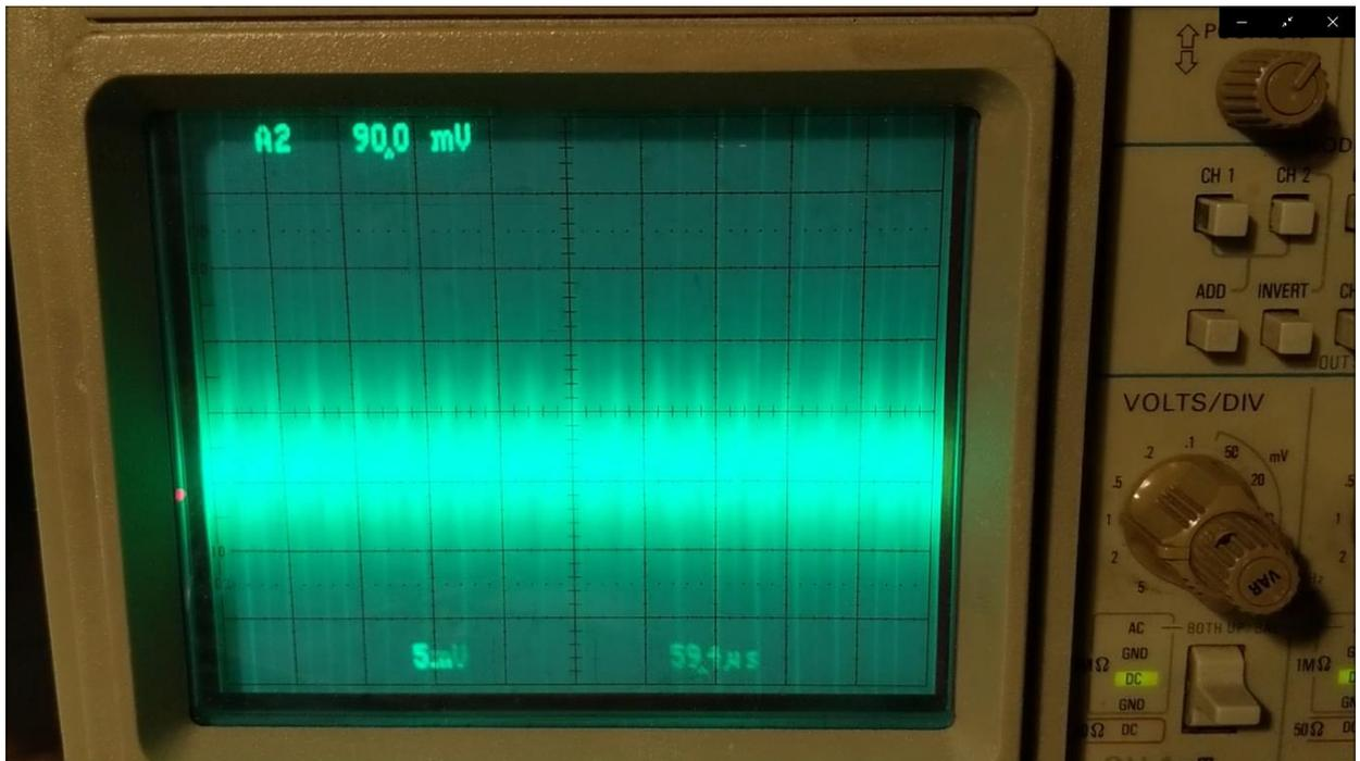
**FIGURE 5:** Oscilloscope readout – 5mV/div, thruster is currently operating in -HV cycle, with corresponding beam reading
