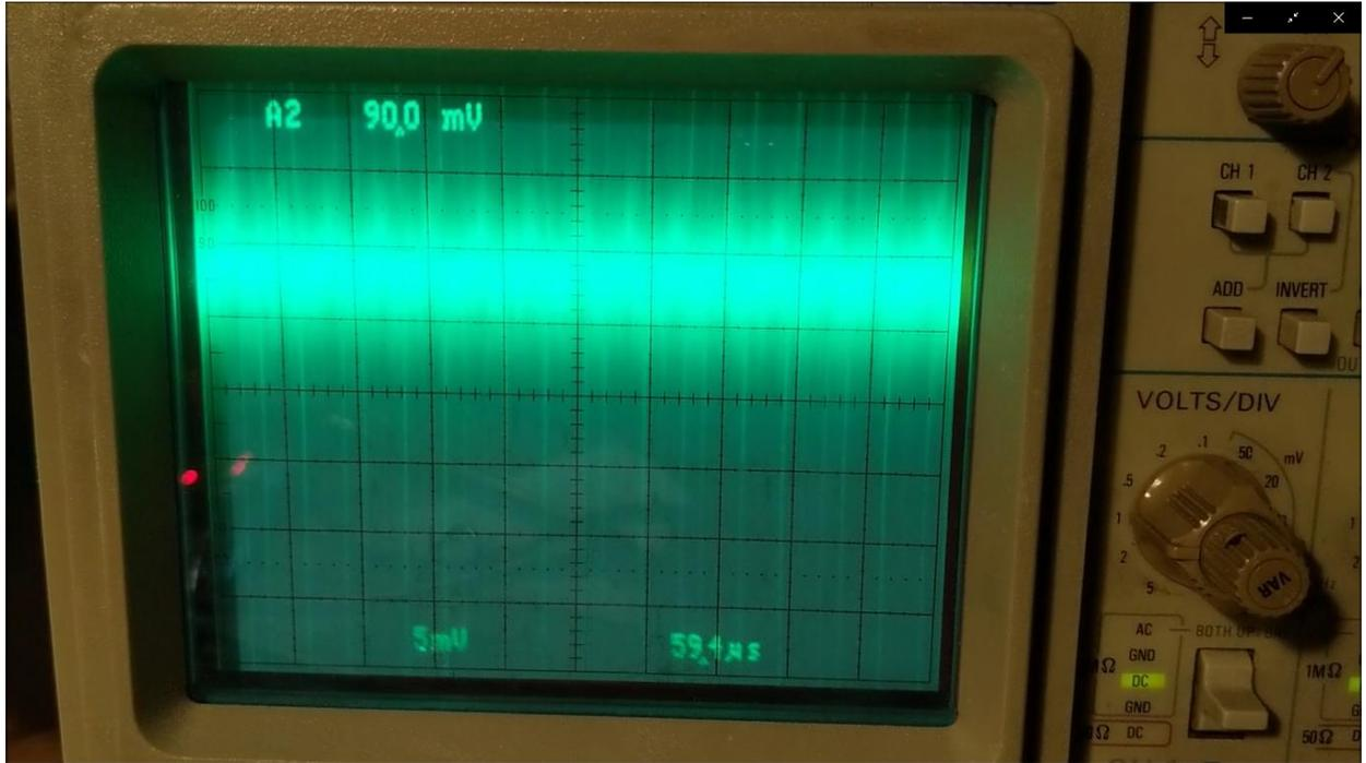
**FIGURE 4:** Oscilloscope readout – 5mV/div, thruster is currently operating in +HV cycle, with corresponding beam reading
