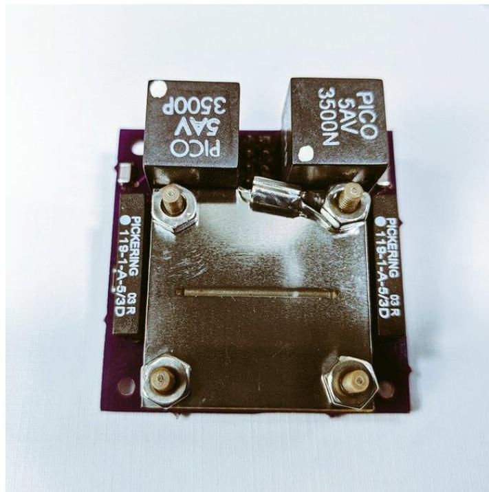
*FIGURE 1: Completed AIS-ILIS1 V6 thruster assembly*
