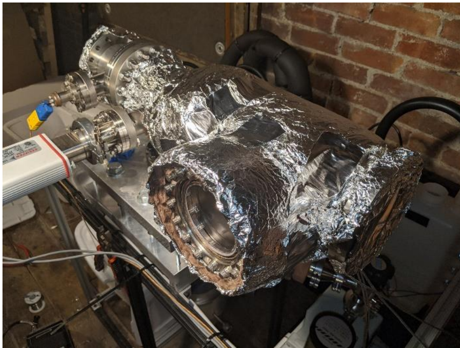
FIGURE 5: Completed TVAC upgrade for thermal cycling and bakeout
