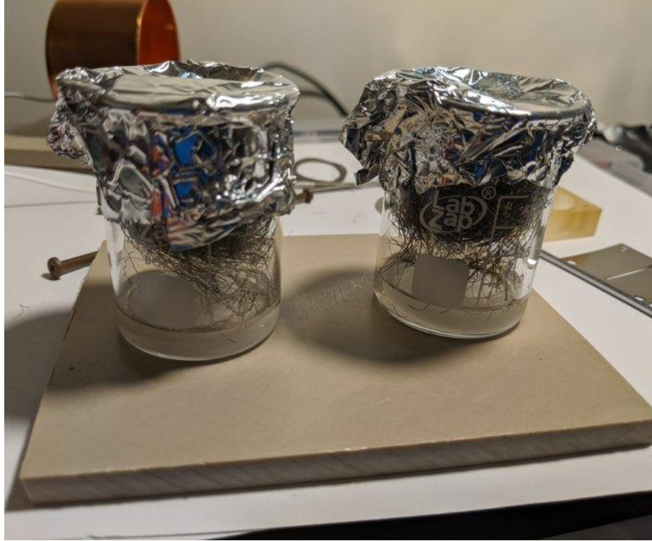
FIGURE 7: Porous glass emitter and reservoir saturated in EMI-BF4
