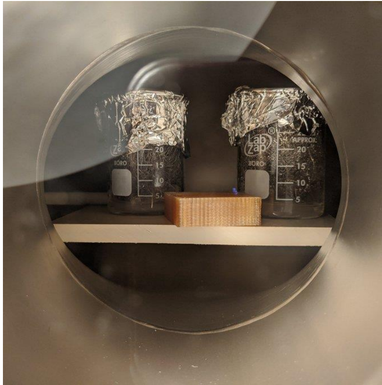
FIGURE 8: Saturated porous glass emitter and reservoir with Ultem housing on PEEK baseplate for baking and degassing
