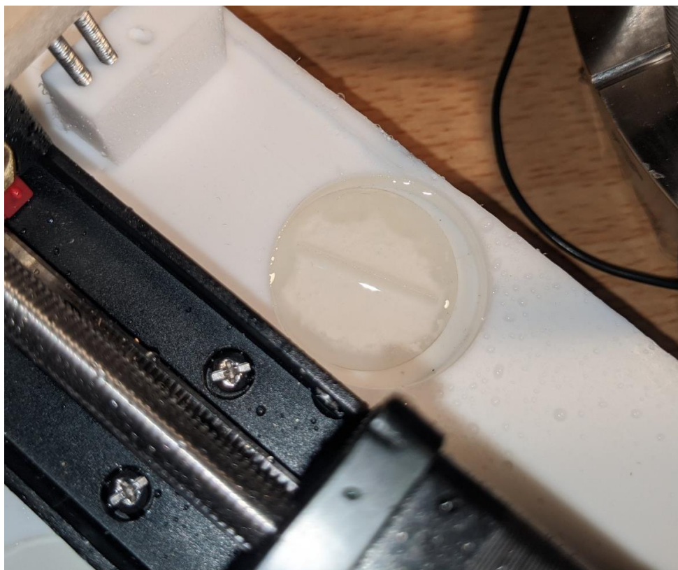
FIGURE 9: Incomplete saturation of the emitter with EMI-BF 4 in atmosphere
