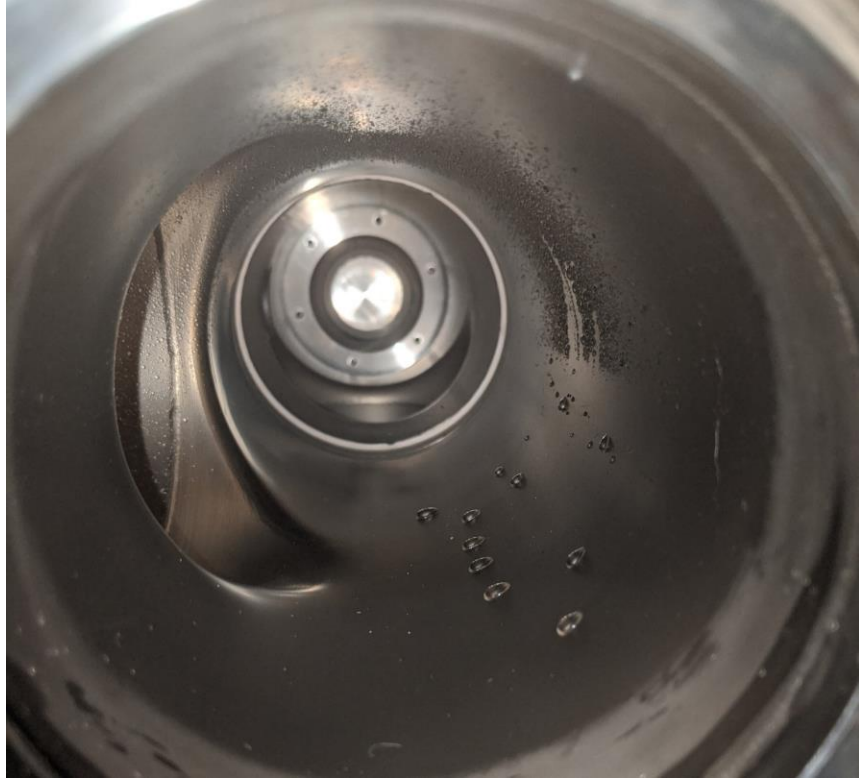
FIGURE 5: EMI-BF4 chamber contamination
