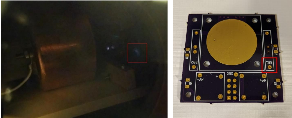
FIGURE 18 AND 19: Ionization fault on board front near +HV relay input pin (LEFT), location of ionization fault on board (RIGHT)
