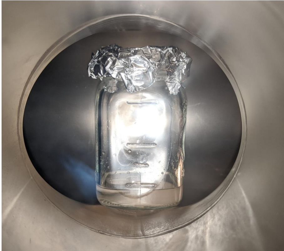
FIGURE 10: Degassing and saturation of emitter and reservoir in vacuum in covered glass container
