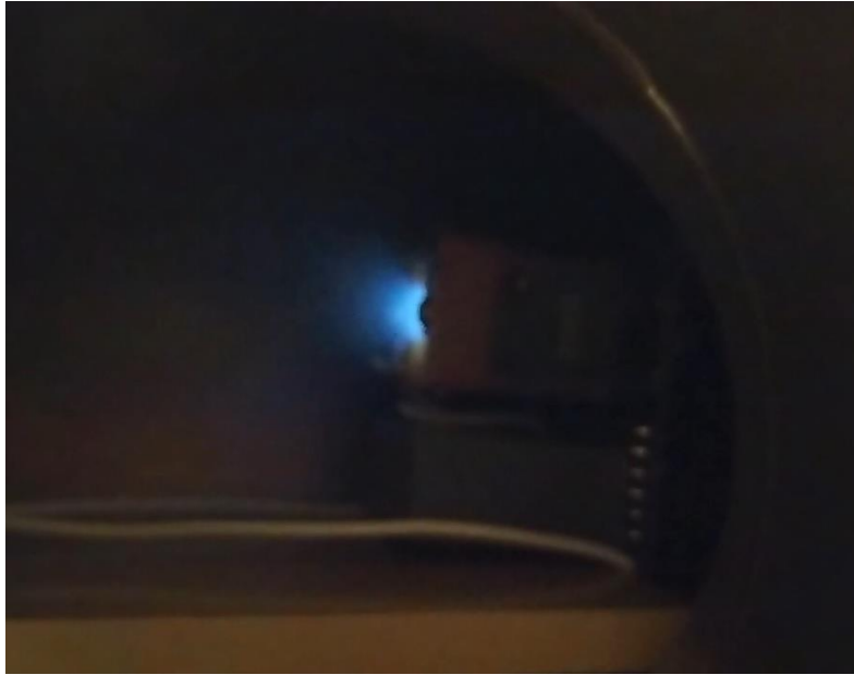
FIGURE 5: Plasma plume resulting from the ignition arc pulse alone. Intensity is significantly higher than all other PPT testing to date due to anode-side triggering.
