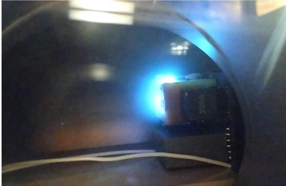
*FIGURE 7: External arc flashover between the igniter connection and anode rail along the outside of the housing.*
