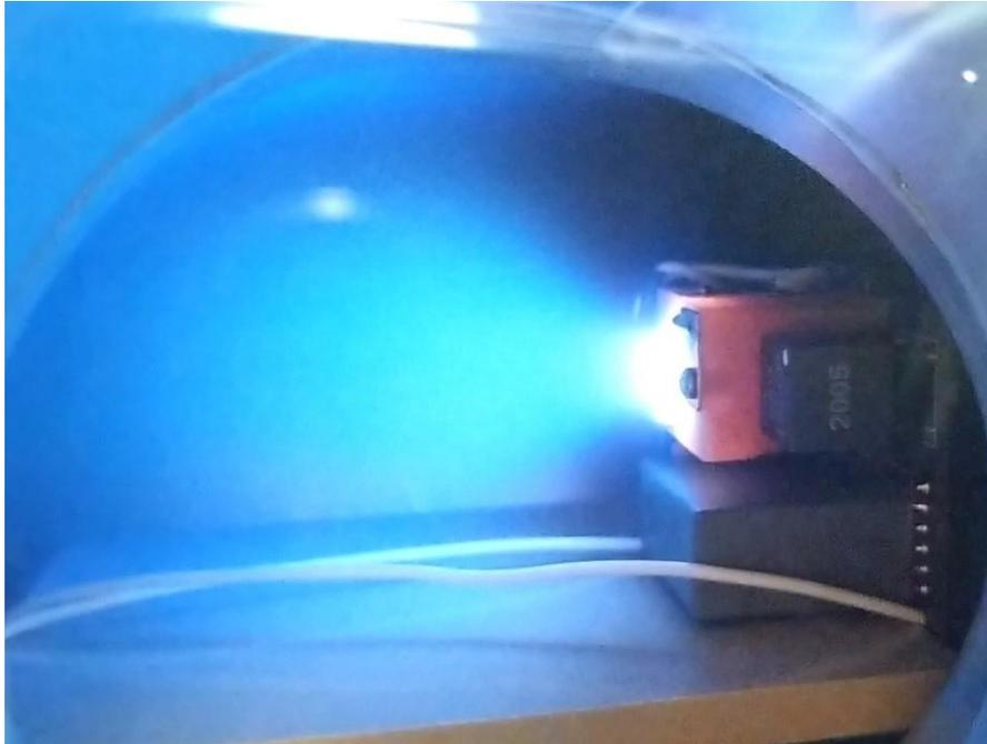
**FIGURE 4:** Successful ignition and firing of the EPPT1 and resulting plasma plume.
