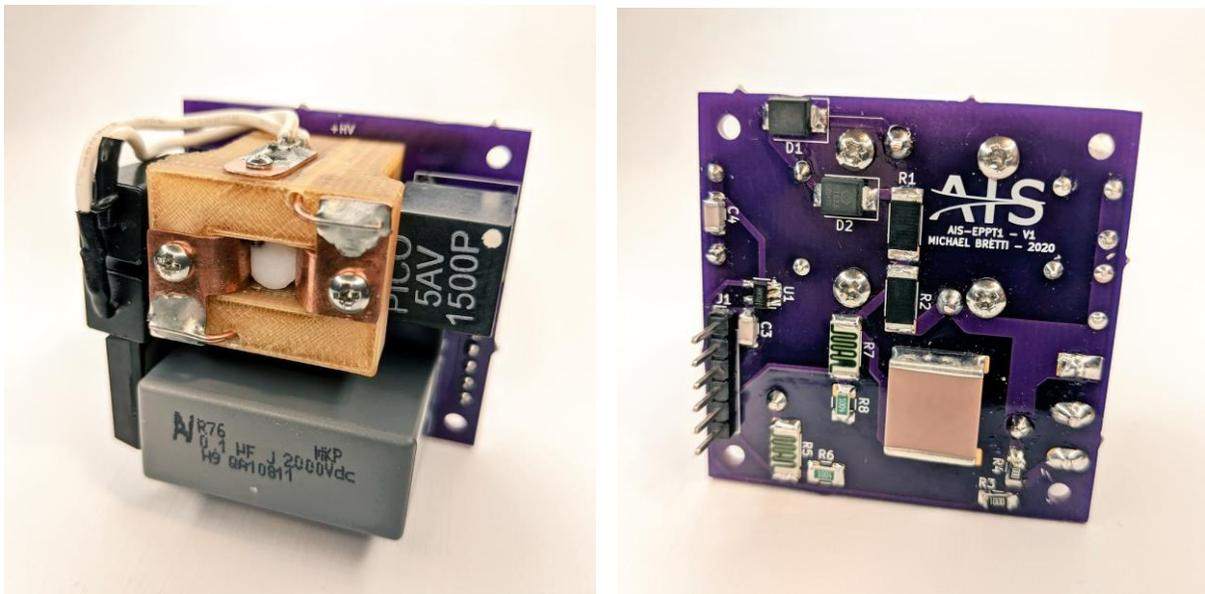
*FIGURE 1: Completed AIS-EPPT1 V1 thruster assembly.*
