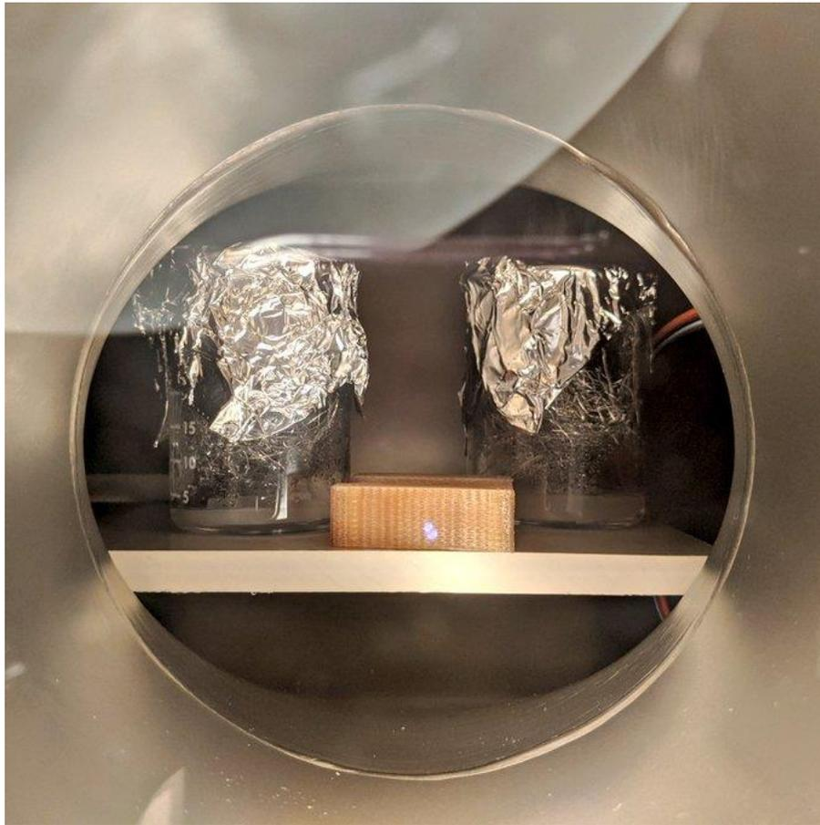
**FIGURE 20:** Saturated porous glass emitter and reservoir with Ultem housing on PEEK baseplate for baking and degassing
