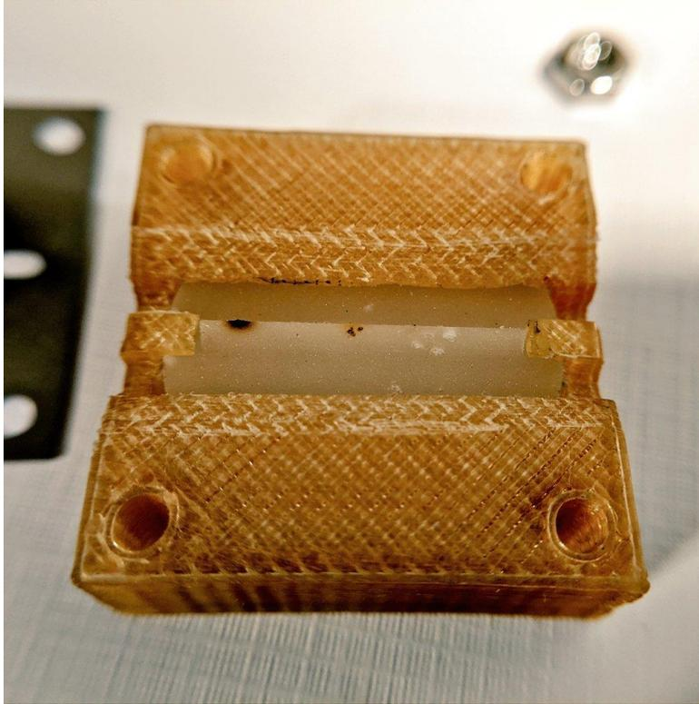
*FIGURE 24: Arcing and fuel deposit on the underside of the extractor*
