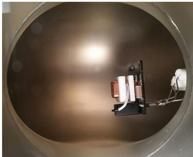
FIGURE 4: AIS-gPPT3-1C V4 thruster centered in high vacuum chamber viewport.
