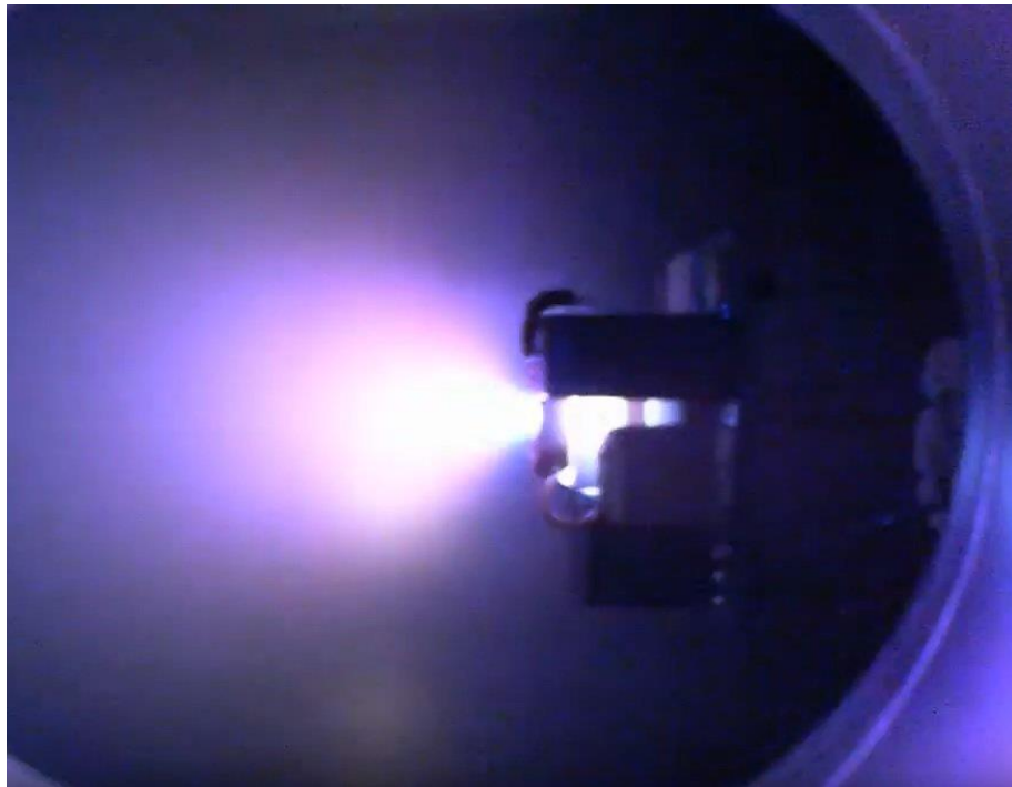
FIGURE 9: AIS-gPPT3-1C plasma plume recorded from webcam during livestream of round 2 lifetime testing.
