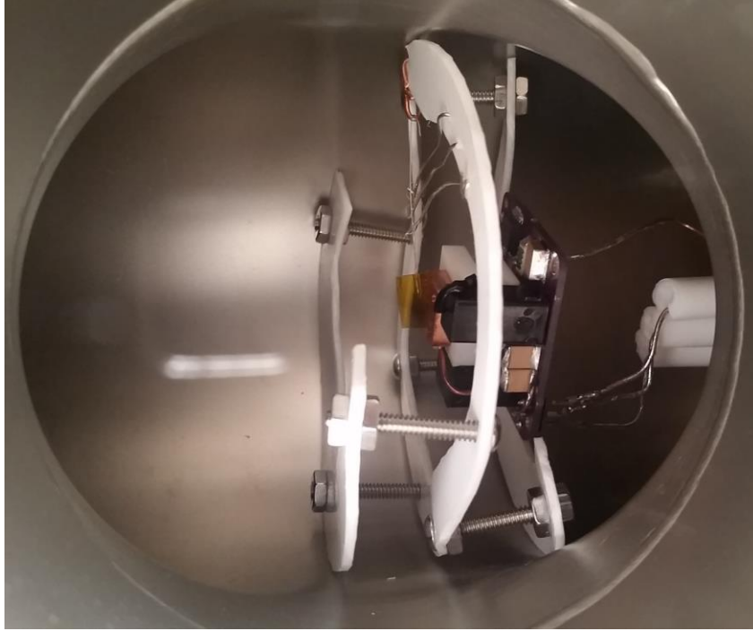
FIGURE 3: Micro-pendulum test stand and AIS-gPPT3-1C mounted into test chamber.
