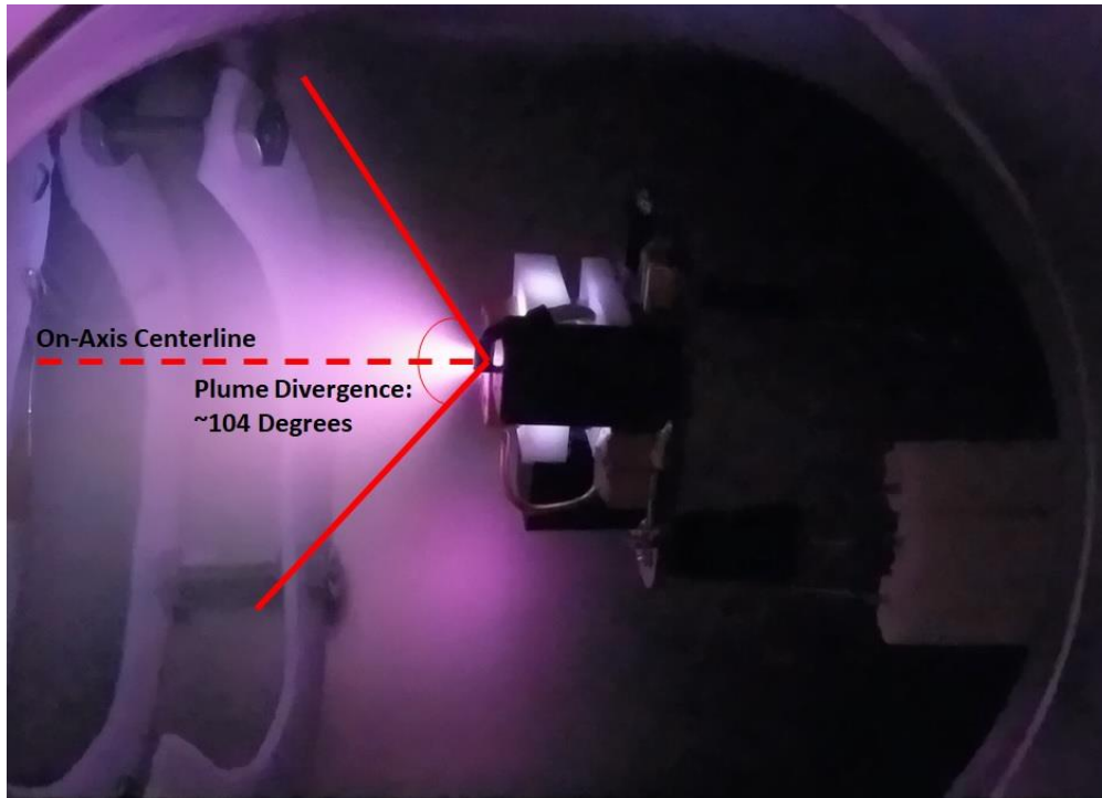
FIGURE 11: Initial plasma plume divergence measurement estimate during successful ignition and firing of the thruster.
