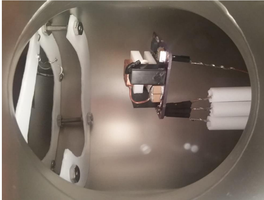
FIGURE 9: View of propulsion module mounted in high vacuum chamber through the viewport.
