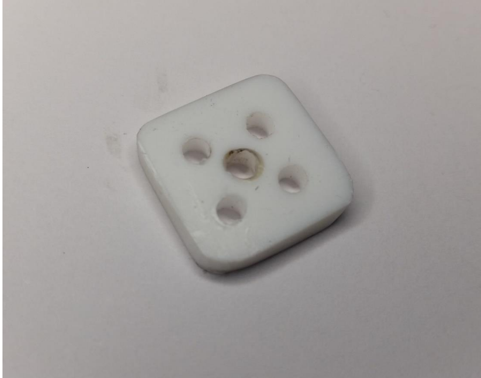
FIGURE 7: Teflon insulator after testing
