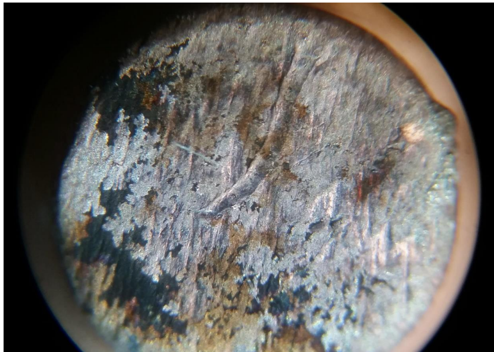
FIGURE 10: Microscopic view of the end of the cathode pin surface after testing
