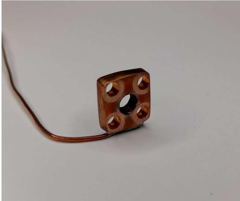
FIGURE 2: Post testing anode
