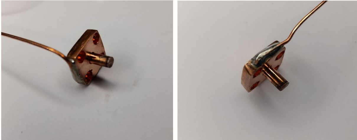
FIGURE 8: Cathode pin surface erosion after testing
