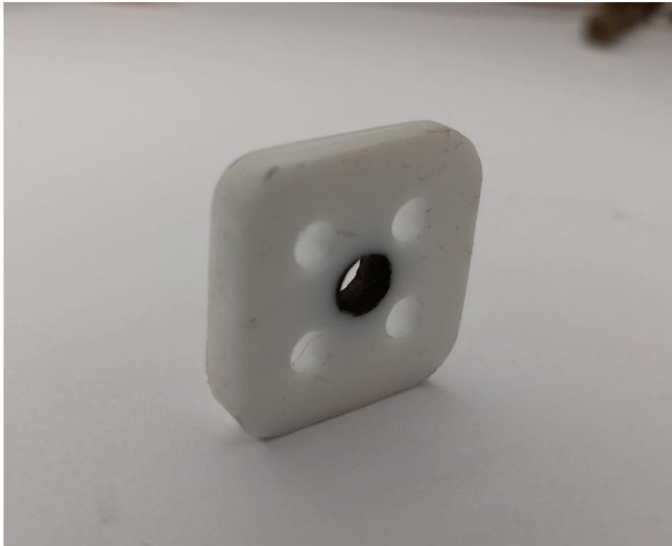
FIGURE 11: Teflon fuel with severely charred bore after testing
