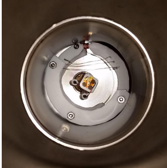
FIGURE 4: Alignment of the micro pendulum Kapton flapper center to the center of the thruster output.
