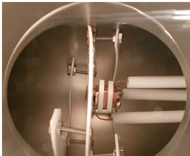
FIGURE 5: Vertical alignment of the pendulum to the thruster, as well as the initial starting distance and captured frame using an external camera for recording.
