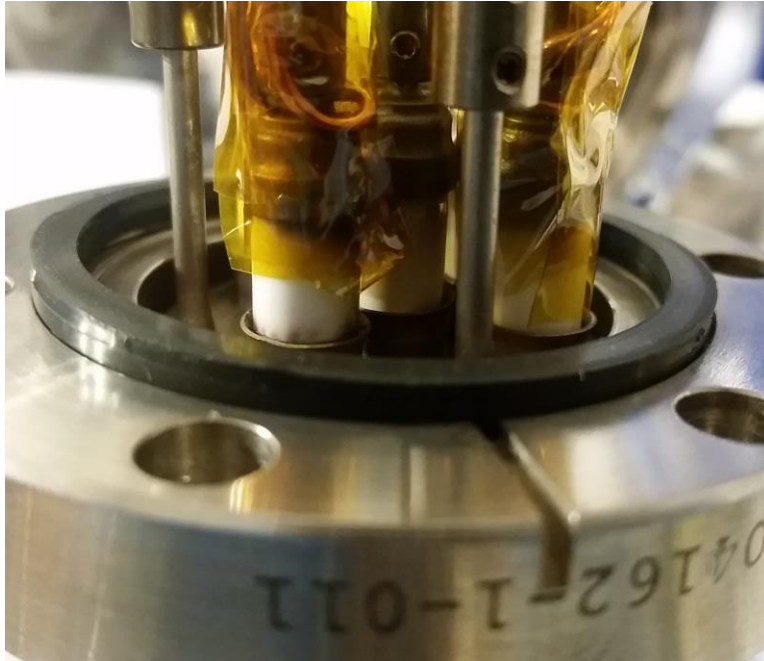
FIGURE 1 – Arcing around ceramic insulators at the base of the conflated feedthrough.
