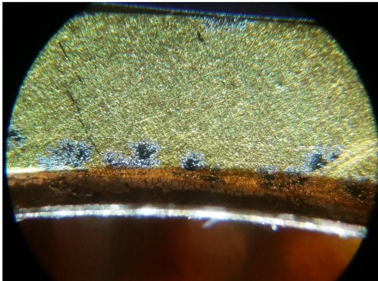
*FIGURE 3 – Cathode board trace ablation from ignition arcs.*
