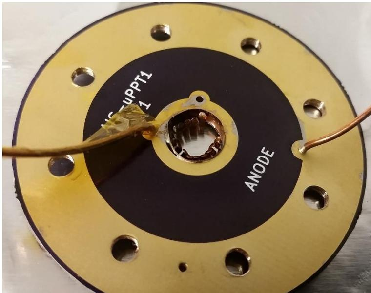
***FIGURE 12 – Ablation of the anode board surface traces due to arcing.***
