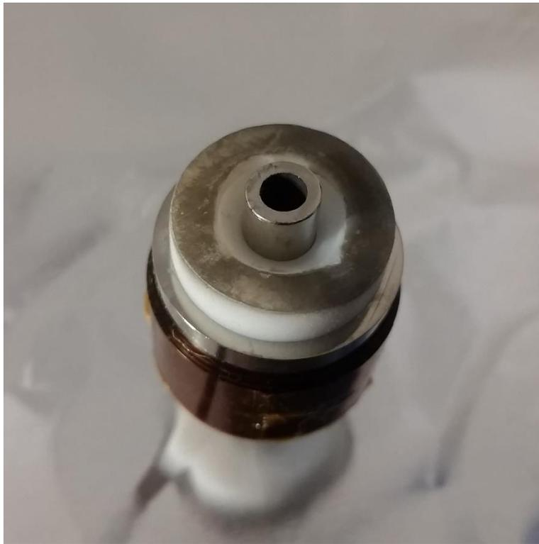
***FIGURE 6 – Teflon fuel charring from ignition on the anode board surface.***
