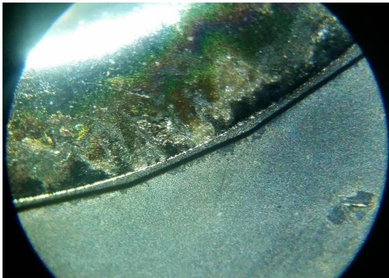
***FIGURE 10 – Charring and ablation of the anode board surface due to ignition of Teflon fuel. Comparison between fingerstock solder trace and the ablated area of the board.***
