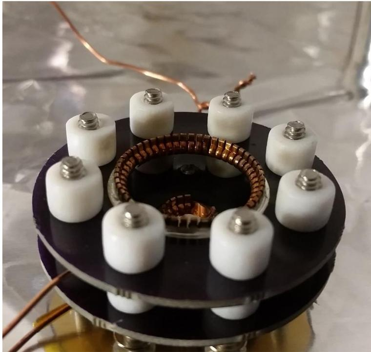
***FIGURE 1 – Cathode-Igniter board Teflon spacer charring due to ignition discharges.***
