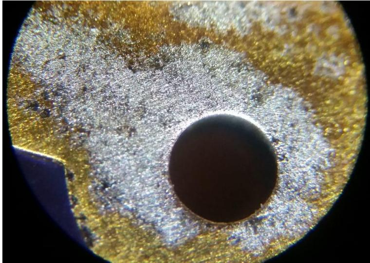
**FIGURE 13 – Microscope picture of anode board surface trace ablation due to arcing. This ablation is present around the arc ignition point identified in Figure 11.**
