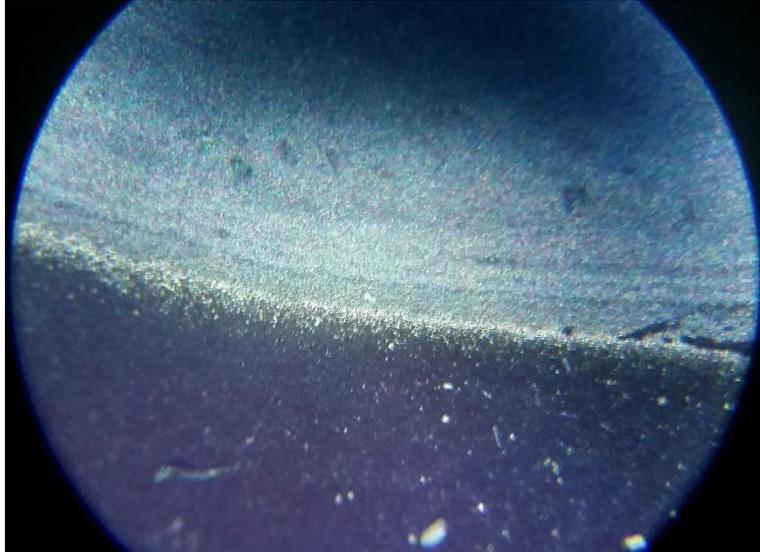
***FIGURE 9 – Charring and ablation of the anode board surface due to ignition of Teflon fuel. Comparison between boundary layer of ablation and normal board surface.***
