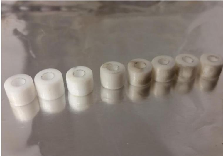
***FIGURE 8 – Charring of the Teflon spacers between the anode and igniter boards.***
