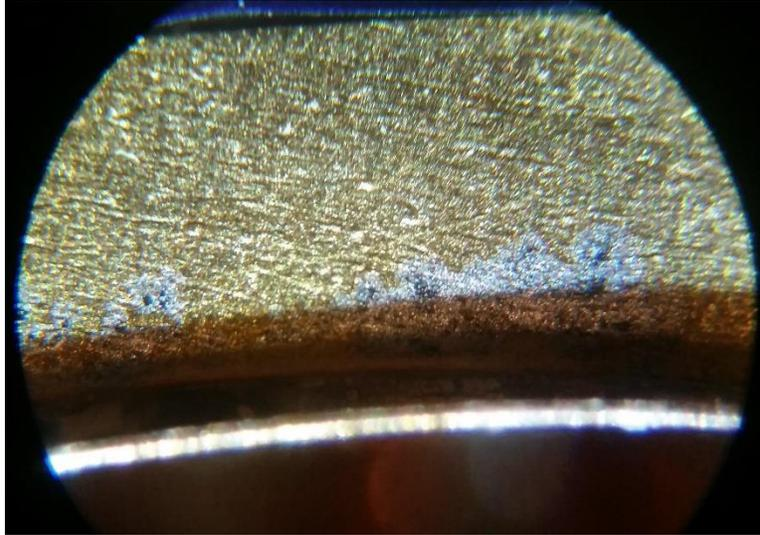
**FIGURE 4 – Cathode board trace ablation from ignition arcs.**
