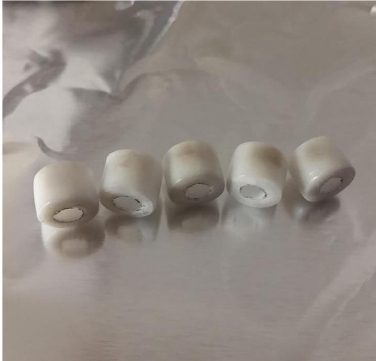
*FIGURE 2 – Cathode-Igniter board Teflon spacer charring due to ignition discharges.*
