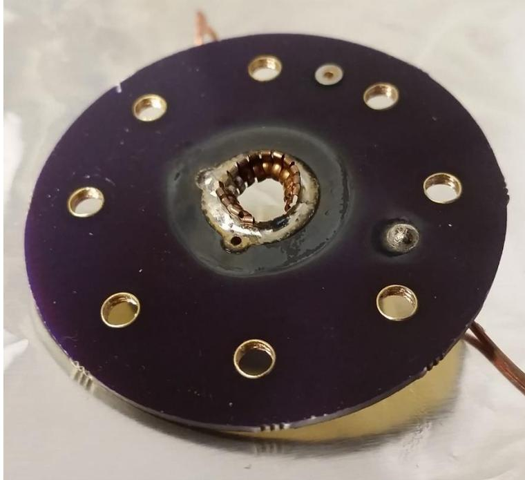
***FIGURE 7 – Charring of the anode board surface due to ablation of the Teflon fuel.***
