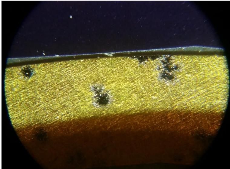
**FIGURE 5 – Cathode board trace ablation from ignition arcs.**
