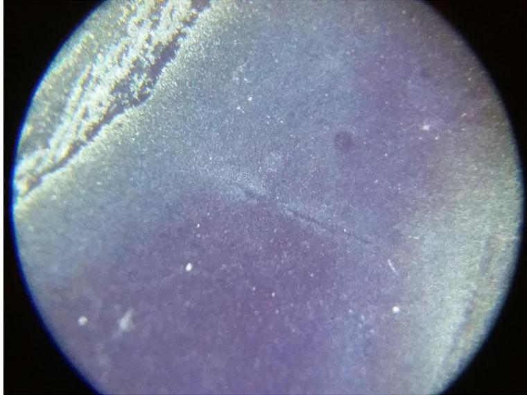
***FIGURE 11 – Charring and ablation of the anode board surface due to ignition of Teflon fuel. Possible arc ignition and formation source between anode fingerstock connection (left) and cathode solder point connection (right).***
