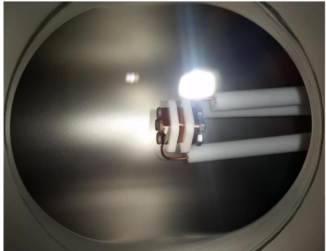
Testing was performed in the Micro Propulsion Testing Chamber using the Integrated High Vacuum Test Stand. Pumpdown conditioning of the system was achieved from atmosphere due to breaking vacuum of the chamber to mount the thruster. Ignition testing vacuum levels were
