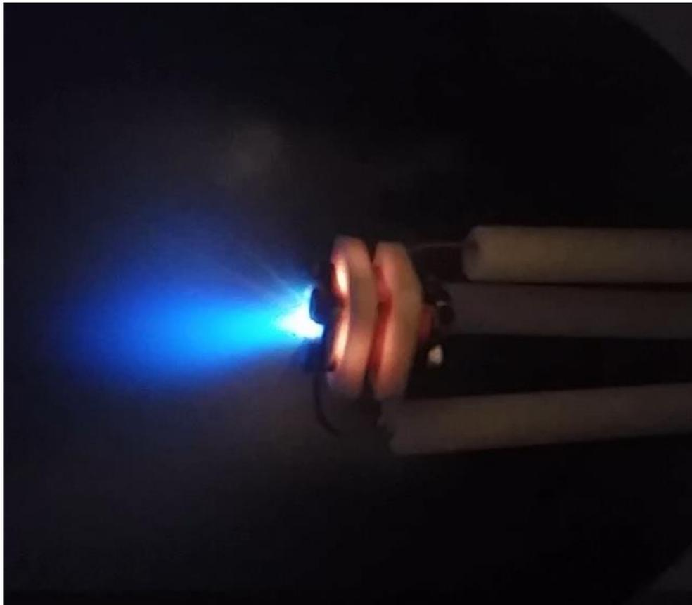
During the total duration of testing, a total of 216 full-power ignitions (0.7J and greater, at over 1kV) were recorded on video, as well as 82 reduced power ignitions at the lower energy (0.23J, 680V), 2Hz repetition rate. This correlates to a total of 298 pulses captured on video. However, the thruster fired numerous times between video recordings, and after the completion of video recording. As a result, it is expected that total ignitions to date is on the order of 350-400.
