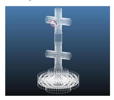
**Simulation 1: Unbaked System, Pumped for <1 Hour** Outgassing Rate (Glass) – 1.333 x 10^-7 mbar\*l/s/cm^2
