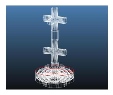
**Simulation 1: Unbaked System, Pumped for <1 Hour** Total Outgassing Load (Viton and Aluminum) – 3.527 x 10^-4 mbar\*l/s
