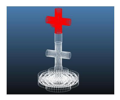
**Simulation 1: Unbaked System, Pumped for <1 Hour** Outgassing Rate (Stainless Steel) – 6.665 x 10^-8 mbar\*l/s/cm^2
