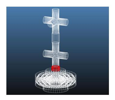
**Simulation 1: Unbaked System, Pumped for <1 Hour** Outgassing Rate (Stainless Steel) – 6.665 x 10^-8 mbar\*l/s/cm^2
