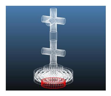
**Simulation 1: Unbaked System, Pumped for <1 Hour** Outgassing Rate (Aluminum) – 1.066 x 10^-6 mbar\*l/s/cm^2
