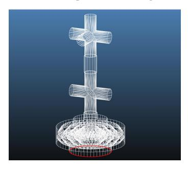
Simulation 1: Unbaked System, Pumped for <1 Hour Pumping Speed – 600 l/s Total Outgassing Load (Viton) – 9.708 x 10^-5 mbar\*l/s
